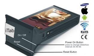
iTab, Remove the double sided tape secure to the base of the MMC avoiding the reset / power on buttons
